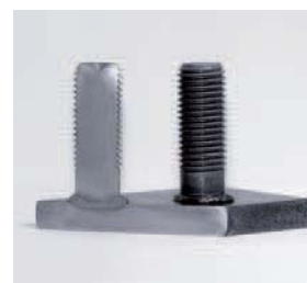
Threaded stud / macro-examination specimen
